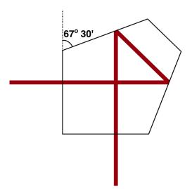
The angle of incidence on the tilted surfaces is  $\theta_{in} = 45^{\circ}/2 = 22.5^{\circ}$  and thus  $\sin \theta_{in} \simeq 0.38$ . This angle has to be equal or larger than the critical angle for which  $\sin \theta_c = n_{out}/n_{in}$ . So we have  $0.38 > \sin \theta_{out} = n_{out}/n_{in} = 1/n_{in}$ , so  $n_{in} > 2.6$ .
